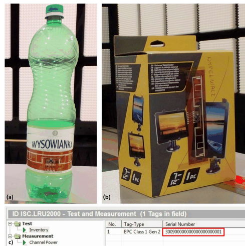
Fig. 9. Transponders under application tests: (a) integration with a PET bottle, (b) integration with a cardboard box, (c) record of the serial number in the RWD application.
