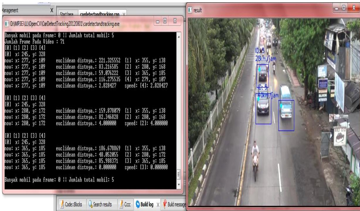
Figure 14. CCTV speed estimation system runs in the background, while vehicles are actually moving in real time
