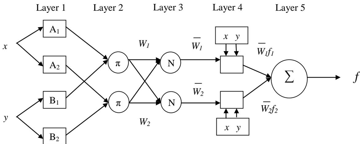
Figure 9. ANFIS algorithm model / architecture
