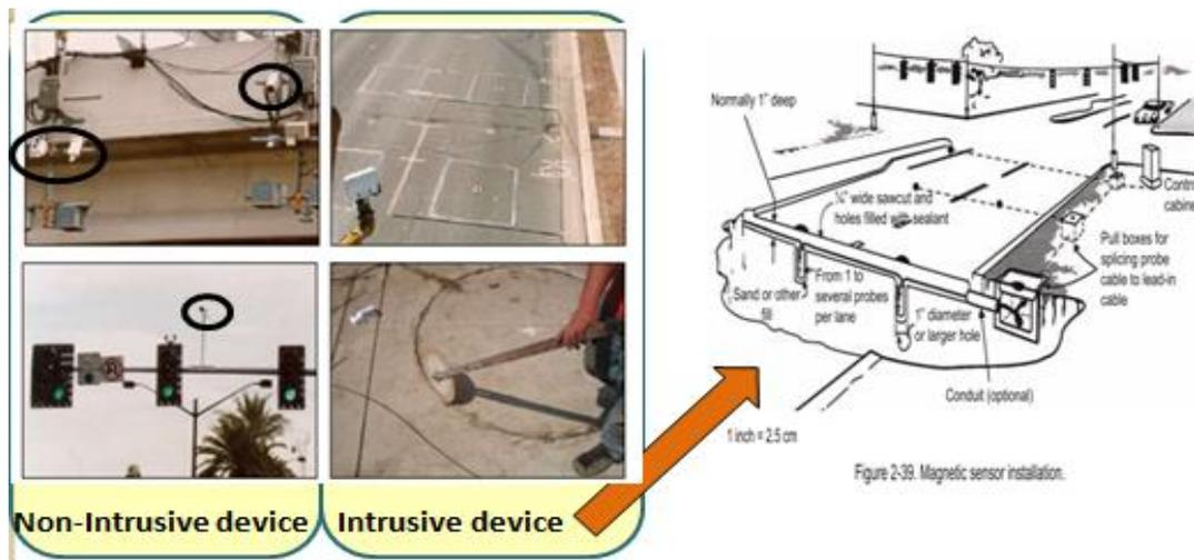
Figure 1. The non-intrusive (e.g. video camera and Radar/Ladar - encircled), and intrusive (e.g. inductive and capacitive/magnetic devices, need to be buried in the road), as traffic sensors, illustration is modified from [2]
