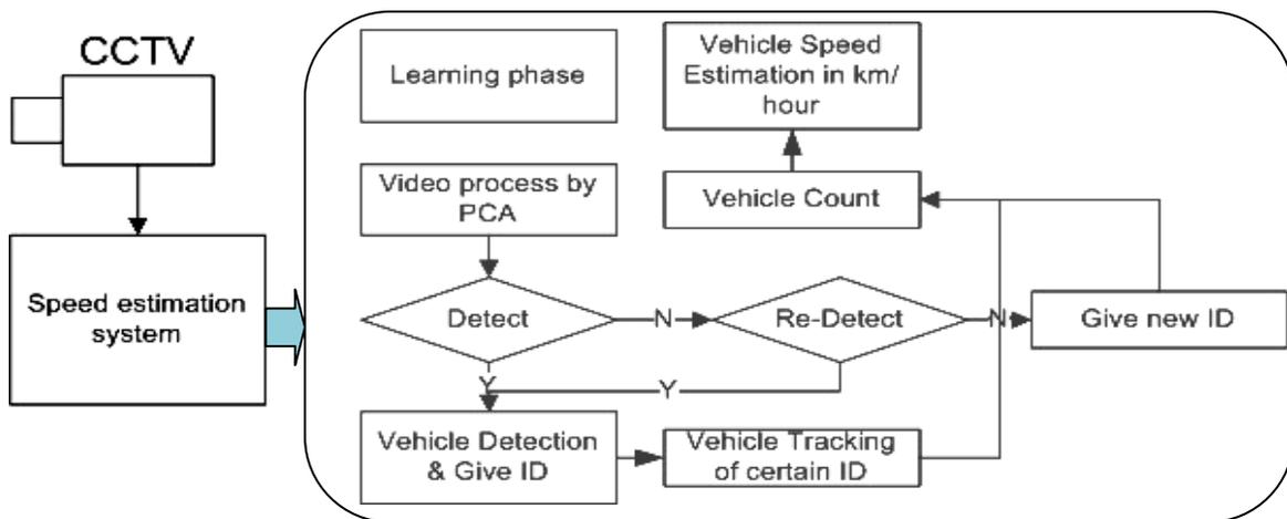
Figure 5. Speed estimation architecture using CCTV employed in our ITS [31]
