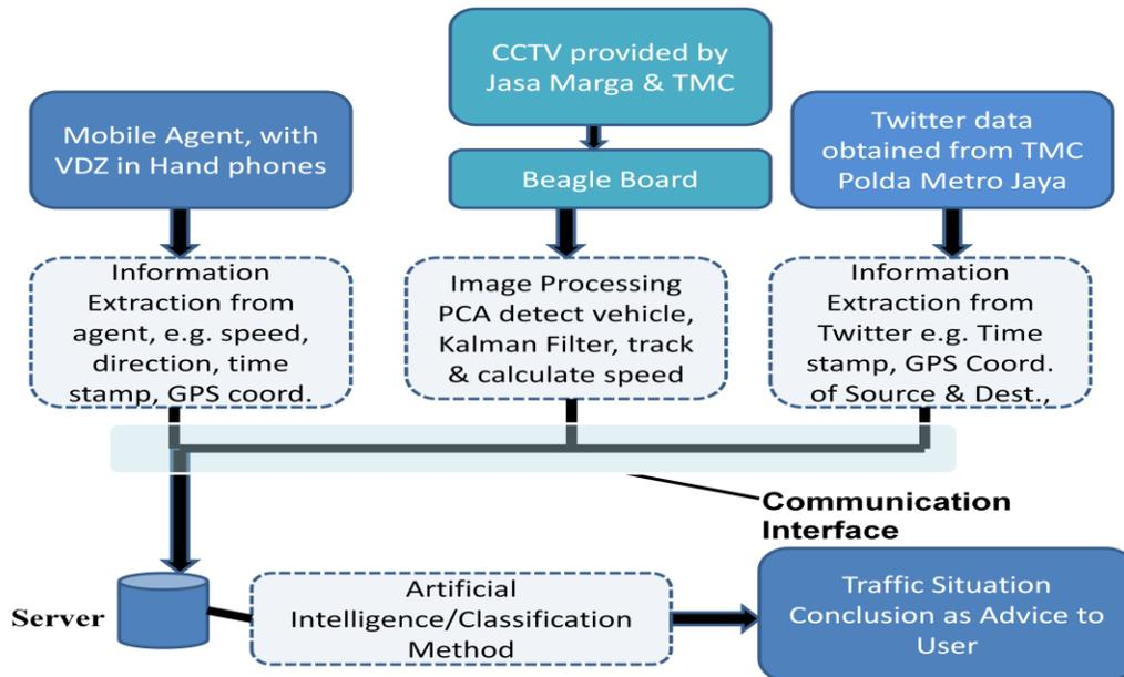
Figure 3. Integrated ITS under Construction at Universitas Indonesia’s Computer Science Faculty.
