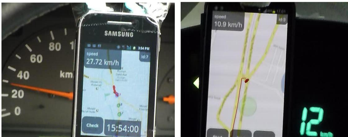
Figure 13. The speeds from GPS data are being compared simultaneously to the speed read from the car's speedometer as Ground Truth (GT) or alternative reference.
