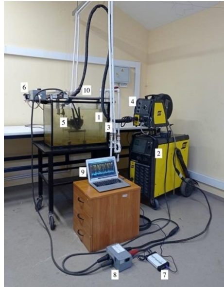
Fig. 2. Underwater cutting setup: 1 – water tank; 2 – source of power; 3 – water supply system and pump; 4 – wire feed system; 5 – submersible stand with sample; 6 – automat of torch movement; 7 – USB-oscilloscope; 8 – current and voltage sensors; 9 – laptop; 10 – torch for underwater cutting
