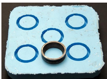
Fig. 1 Silicone mold for making composite rotating ring
