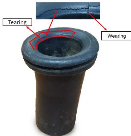
Fig. 1. Damaged textile machine yarns pass analyzed
