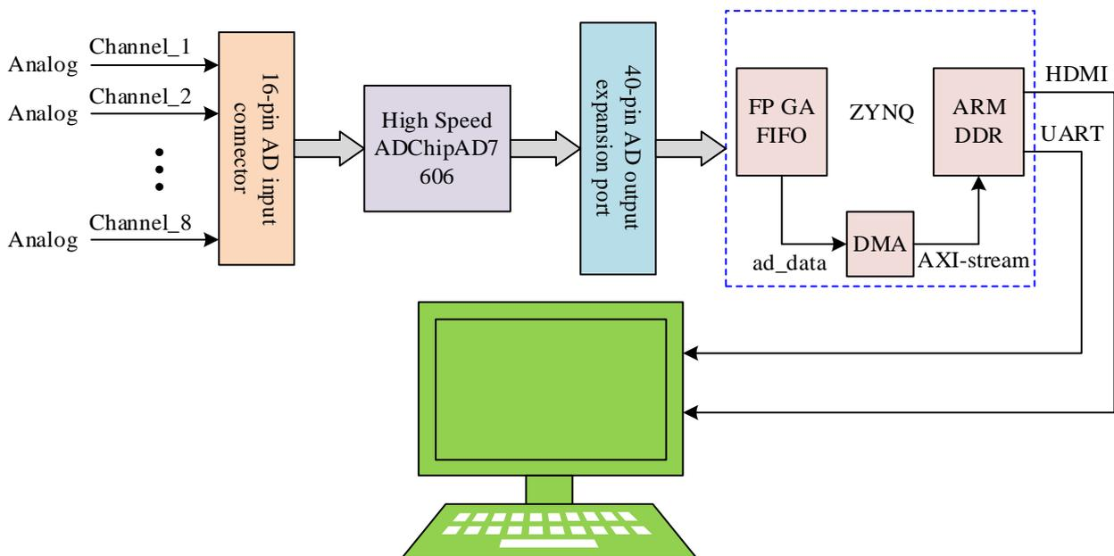
**Figure 1.** The overall design of the data acquisition system
