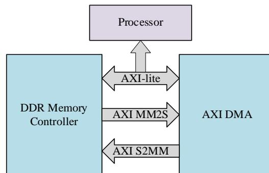
**Figure 2.** Chip internal data transmission
