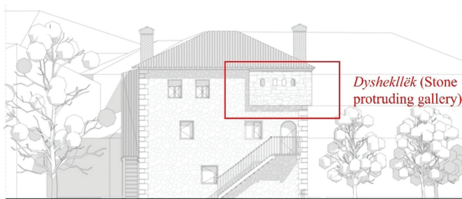
Fig. 4. Dyshekllek (protruding stone gallery) in the Kulla of Isuf Mazrekaj in Dranoc, Kosovo [drawing by authors].
