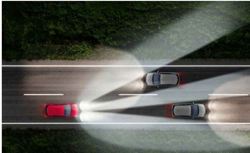
Fig. 1 – Adaptive headlamp with Matrix Manager devices.
