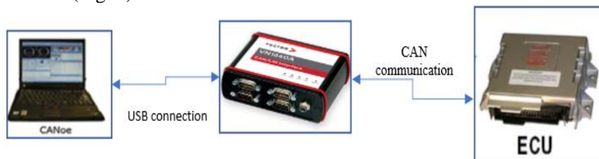
Fig. 3 – ECU to USB Connection.
