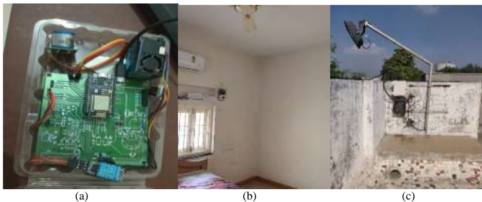
Fig. 5. Prototype (a); deployment at home(indoor) (b); deployment rooftop (outdoor) (c)
