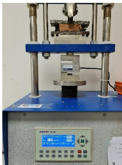
Fig. 10: Set-up of compressive test.
