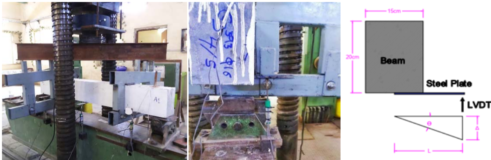
Fig. 3: Deflection and rotation measurement.
