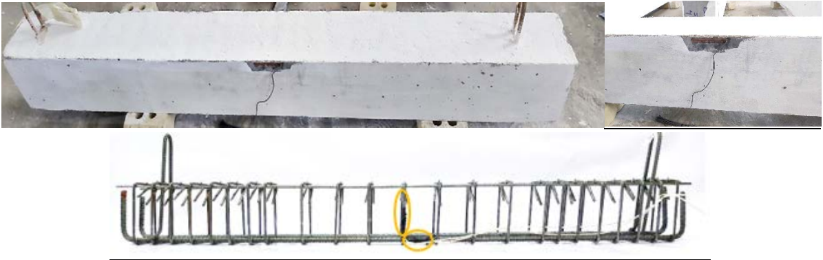
Fig. 1: Placement of strain gauges.
