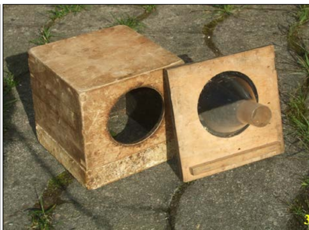
Figs 1-3: Wooden elector for obtaining all insects during sweep net fieldwork. The net content is emptied through the opening above, the funnel should be orientated towards the sun or lightest area of the sky. Construction by MvT.
