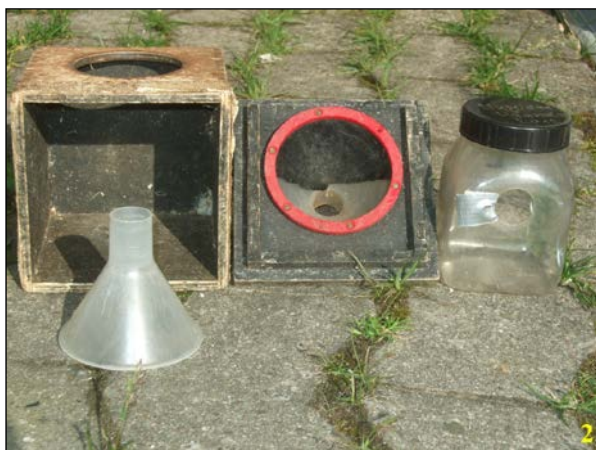
Figs 1-3: Wooden elector for obtaining all insects during sweep net fieldwork. The net content is emptied through the opening above, the funnel should be orientated towards the sun or lightest area of the sky. Construction by MvT.
