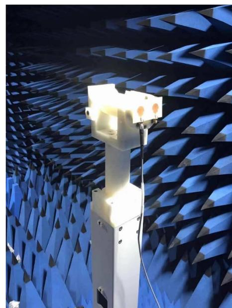
Fig. 9. Far-field measurement setup.
