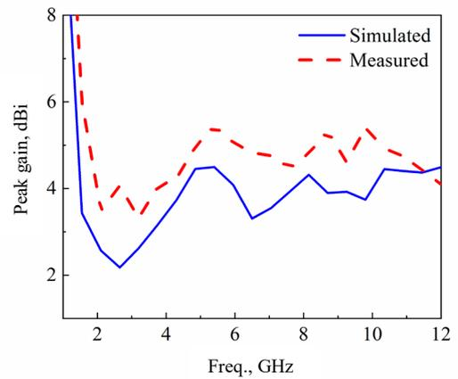
Fig. 8. Measured and simulated peak gain.
