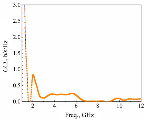
Fig. 13. CCL of UWB/MIMO antenna system.
