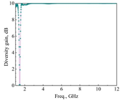
Fig. 14. Diversity gain of UWB/MIMO antenna.
