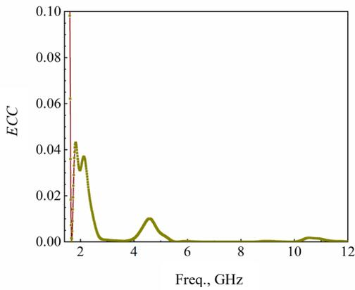
Fig. 12. ECC of UWB/MIMO antenna system.
