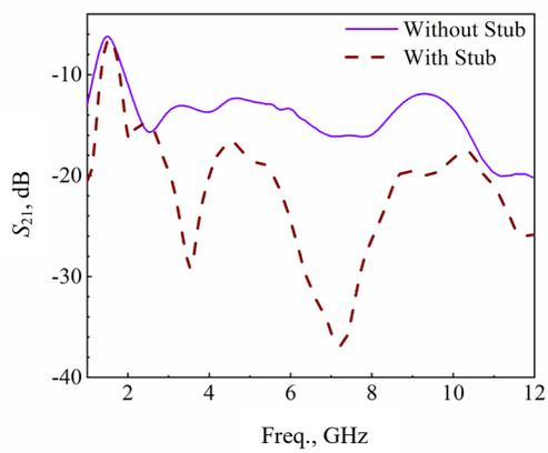
Fig. 6.  $S_{21}$  without and with a stub.
