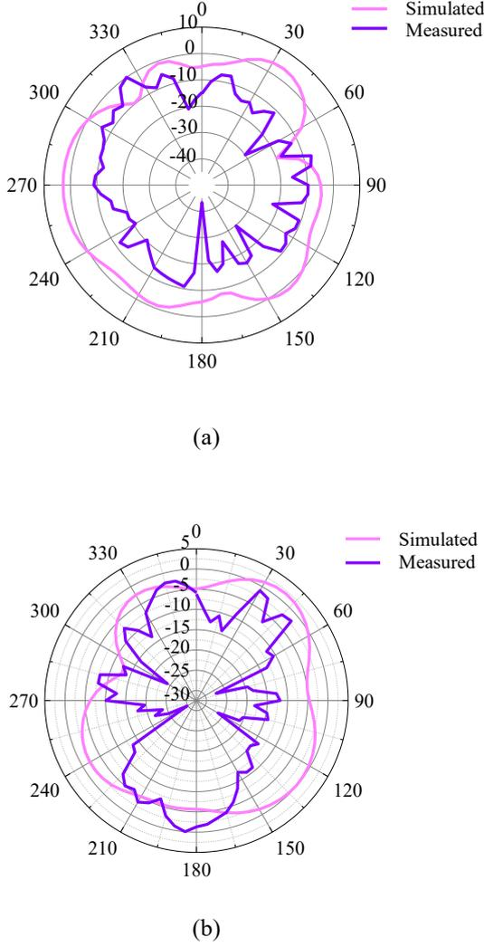
Fig. 10. Measured and simulated directivity for (a) E-Plane, (b) H-Plane at 10.6 GHz.
