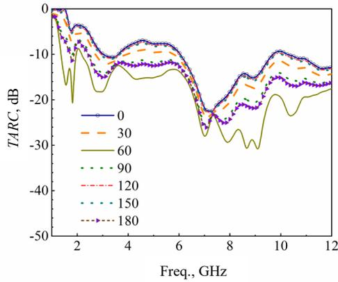
Fig. 11. TARC of the MIMO antenna system when  $\Theta$  changed from  $0^\circ$  to  $180^\circ$ .
