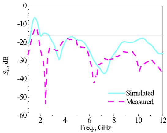
Fig. 4. Measured and simulated  $S_{21}$ .
