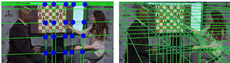
Figure 12. Visual differences between our algorithm (right) and the method by Danner and Kafafy [10], which utilizes a single Hough transform without segment merging (left). One can see that our method generates much more information from an image, which can later be utilized to find lattice points and localize a chessboard.
