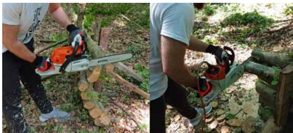
Fig. 2. Vibration measurement on the chainsaws used in late cleaning.
