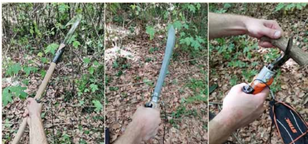
Fig. 1. Vibration measurement on the tools used in early cleaning.
