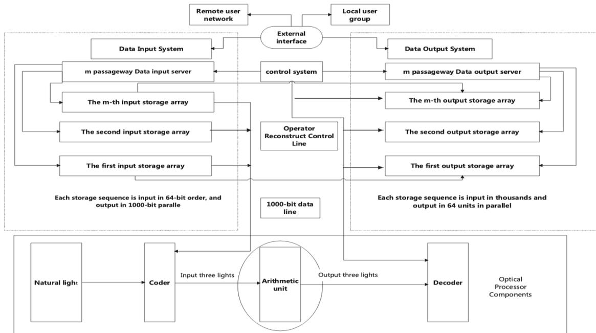
Figure 1. Conceptual diagram of ternary light computer
