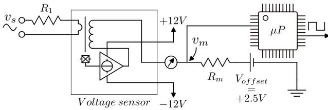
**Fig. 3.** A general structure of the voltage sensor with  $\mu\text{P}$ -based ZCD circuit
