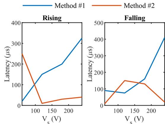
**Fig. 7.** Latency (delay/haste) in detecting the ZCPs using Method #1 and Method #2
