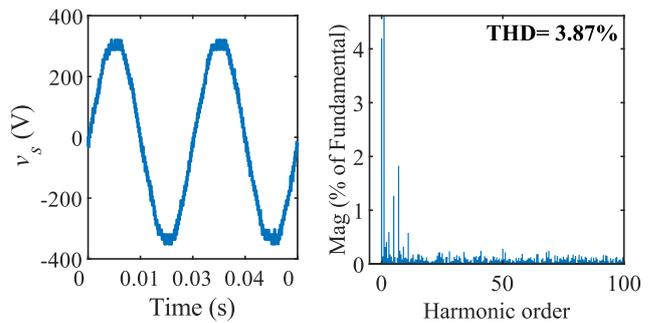
**Fig. 5.** Source input voltage waveform and its harmonics
