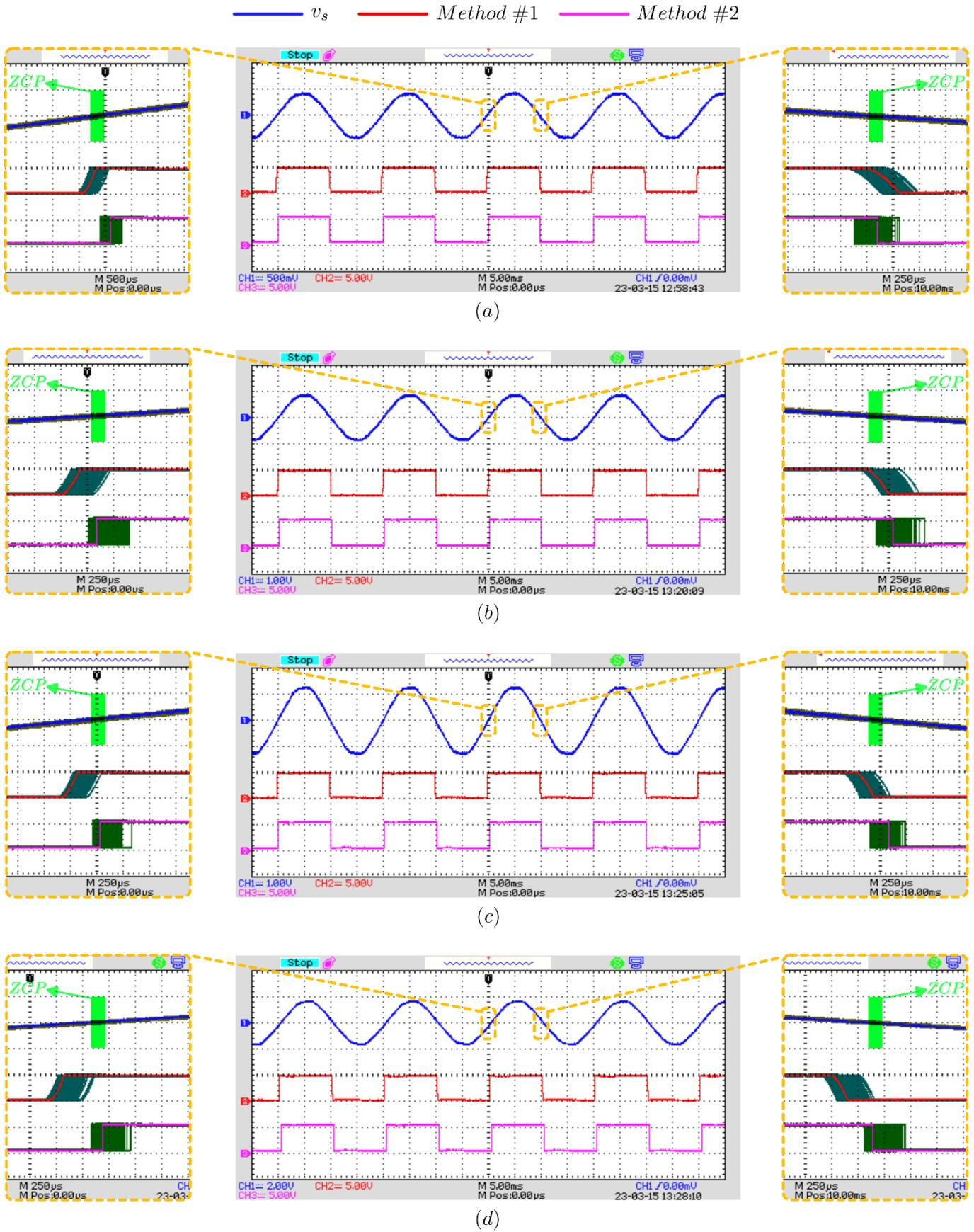
**Fig. 6.** ZCD signals obtained using Method #1 and Method #2 at source voltages (a) 60  $V_{rms}$ , (b) 120  $V_{rms}$ , (c) 180  $V_{rms}$ , and (d) 240  $V_{rms}$
