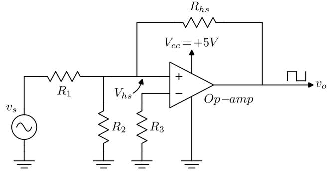
**Fig. 2.** A general structure of the op-amp-based ZCD circuit with resistive feedback hysteresis
