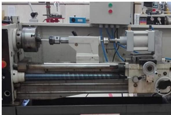
Fig. 1. CDFW machine setup. CDFW, continuous drive friction welding
