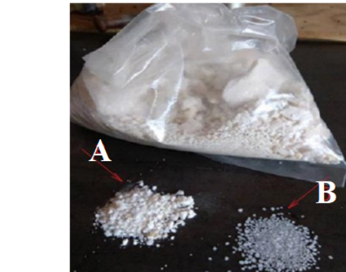
Fig. 5. Aluminum sulfate: sample A – first grade; sample B – top grade
