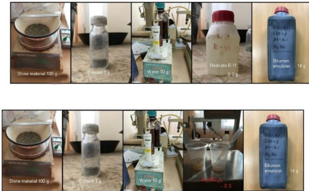
Fig. 7. Components in cast emulsion–mineral mixtures
