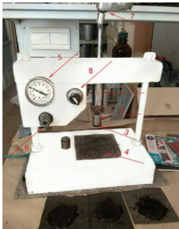
Fig. 9. Modified cohesive device: 1 - air cylinder; 2 - cylinder rod; 3 - rubber tip; 4 - a plate of roofing felt(s); 5 - pressure gauge for measuring the pressure in the cylinder; 6 - air pressure regulator; 7 - torque wrench; 8 - regulator for lowering the cylinder rod
