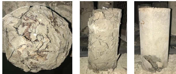
Fig. 6. Destroyed concrete specimen from 500°C exposure
