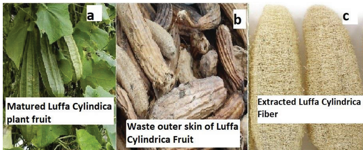
Fig. 1. Digital image of (a) Mature Luffa cylindrica plant fruit; (b) waste outer skin of Luffa cylindrica fruit; (c) extracted Luffa cylindrica fibre
