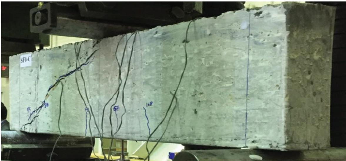
Fig. 4. Failure pattern of specimen DB-NS0
