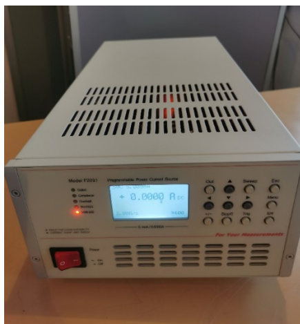
Fig.3. Programmable Controlled Power Supply DX-F2031 for the electromagnet.
