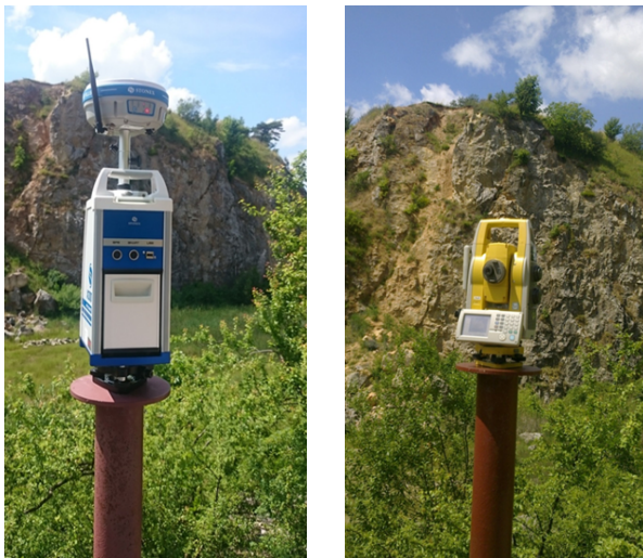
(a) Satellite techniques combined with a laser scanner (b) Total station surveying
