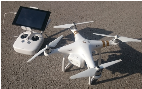
(c) Photogrammetric technique using a UAV (Krawczyk, 2021)
