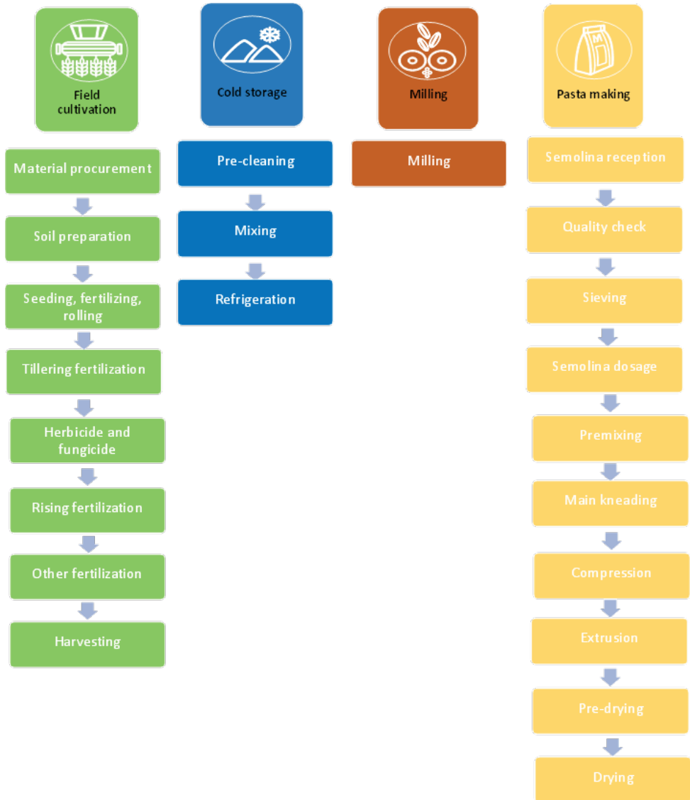
Fig. 1. System boundaries of the system.
