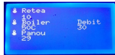
Figure 16. Display of results on LCD 128*64 pixels – case of temperature 3-50°C
