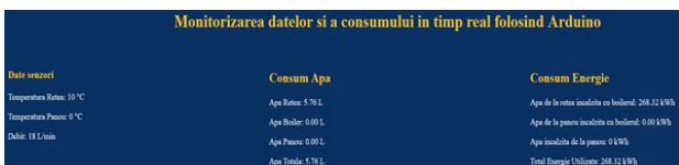
Figure 19. Data acquisition when the water in the panel is between 0° and 3°C and the water flow is greater than 0
