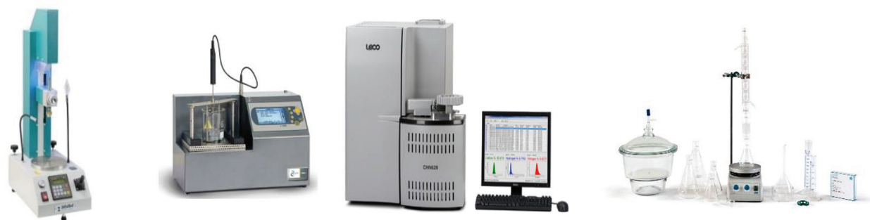
Fig. 4 Equipment for the tests performed (from the left: penetration, softening point, elementary analysis, group analysis)
