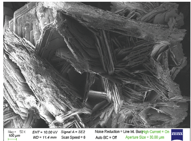
Fig. 9 Microstructure of the calcium carbonate precipitation ( \text{CaCO}_3 ) on the BC samples at 200X magnification.
