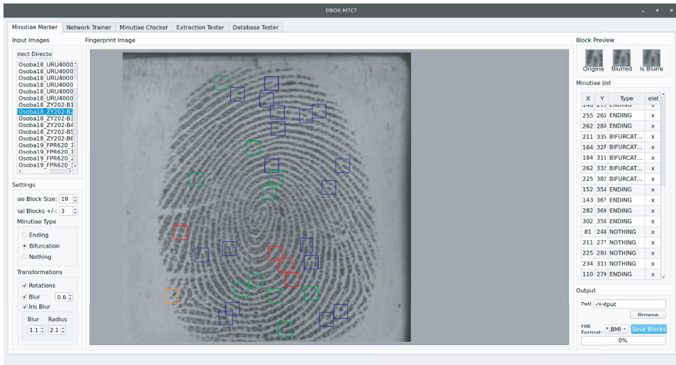
FIGURE 9. User interface of the application for training data collection depicting minutiae marking.
