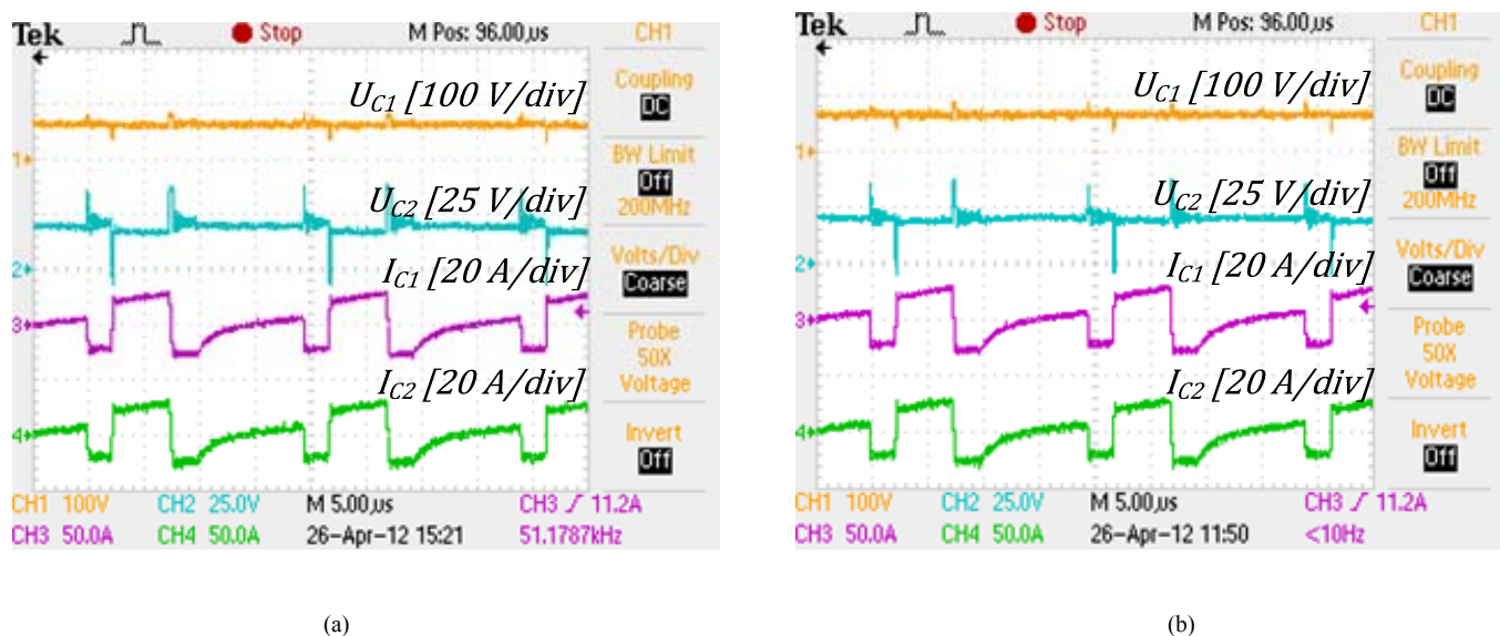
Fig. 7. Operation waveforms ( U_{C1} , U_{C2} , I_{C1} , I_{C2} ) of a qZSI with electrolytic capacitors (a) and with ceramic capacitors (b) at U_{in}=40 V.
