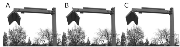
Fig. 8. Location of keypoints for charger pose estimation: four points located on the head and called head (a), four points located on the natural corners of the head and the mast, called corners (b), and four points located inside the artificial markers, called markers (c).
