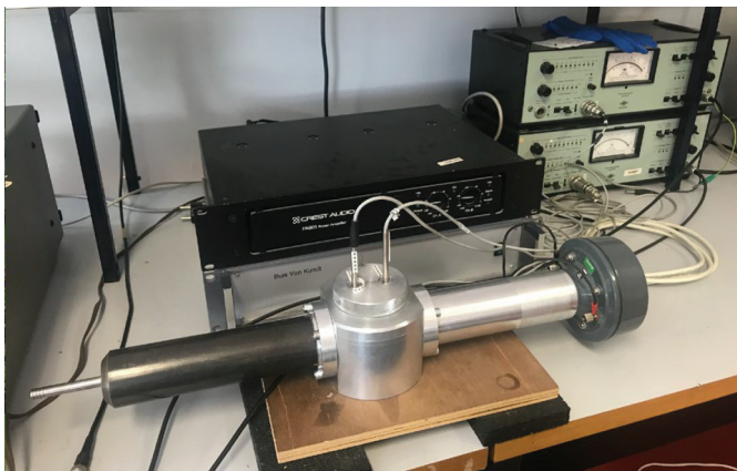
Fig. 2 Measurement set up: impedance tube
